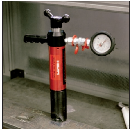
Pull-out test of an ENP fastening with a HAT28 tester and X-ENP adapter
