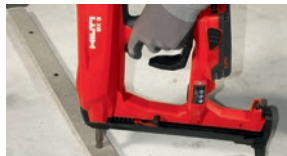
Fastening wood, e.g. Placopan®, to concrete
